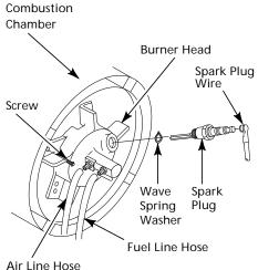
Figure 16 - Removing Burner Head
